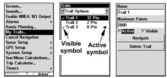
Sequence for saving a trail and beginning a new one. My Trails command (left). The Trails Menu (center). The arrow to the right of Trail 3 indicates the trail is active and the check to the left indicates the trail is visible on the map display. The Edit Trail menu (right) with the Name command selected.
